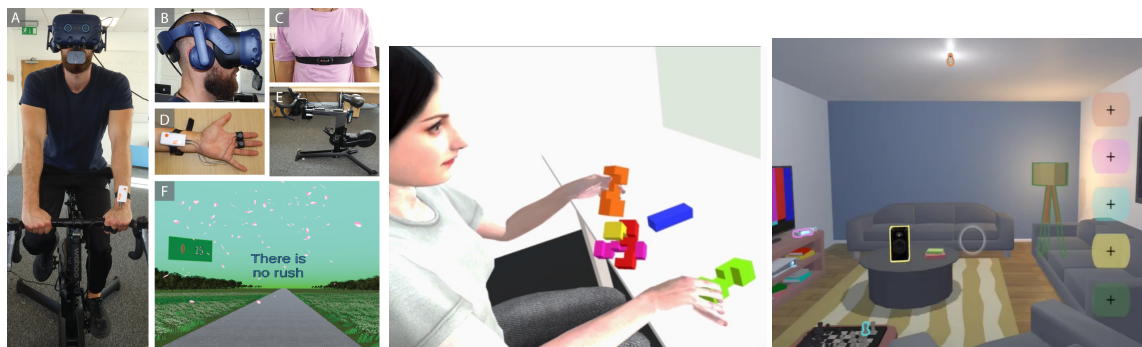
Figure 1: Left (A-F): In our affective VR exergame, a user wears sensors such as a face tracker (B), a heart rate strap (C) and skin conductivity electrodes (D) while riding a stationary exercise bike (E) through emotion-inducing virtual environments (F). Middle: Our virtual learning environment for psychomotor tasks teaches users to complete a 3D Burr puzzle through observational learning (watching an avatar) or active learning (guided practice). Right: Users control a virtual smart home through eye gaze, e.g. activating a smart speaker or switching off lights by dwelling on colour-coded dwell buttons in their periphery.
