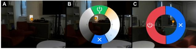
**Figure 8: A: The user invokes an Radi-Eye interface for appliance control by gaze dwelling on an appliance. B-C: The object-dependent interface adapts to the selected appliance (B: lamp, C: fan) and is centred around the user's head.**
